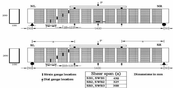
Fig.1. Test setup and strengthening scheme (CFRP strips in the form of U-WRAP)
