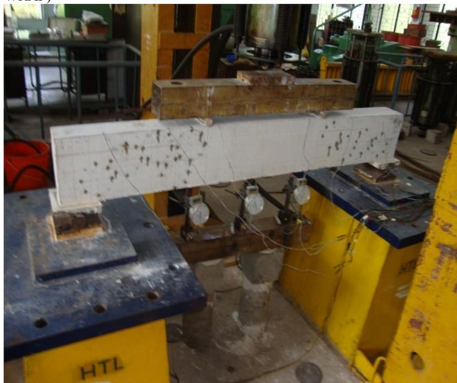
Fig. 2 Two points loading experimental arrangements for control beam
