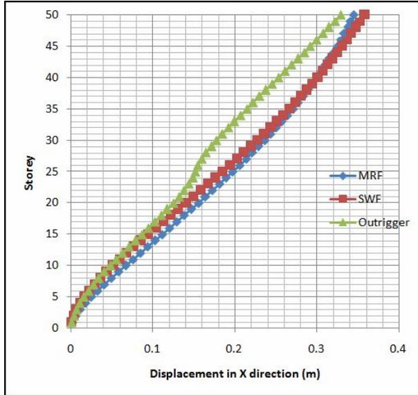
Fig. 11. Storey displacement variation along height in X dir.
