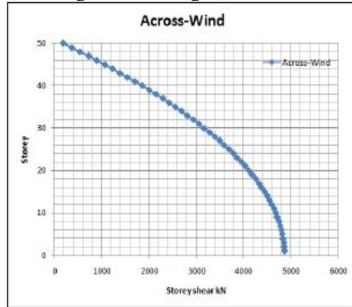
Fig. 2. Storey shear considering across wind loading
