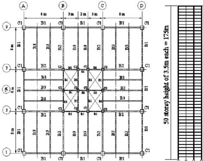
Fig. 3. Moment Resisting Frame (Typical floor plan and elevation)
