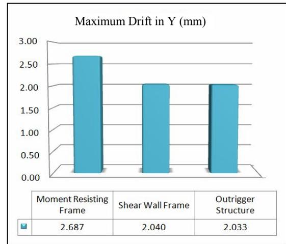
Fig. 10. Comparison of Maximum storey drift in Y dir.
