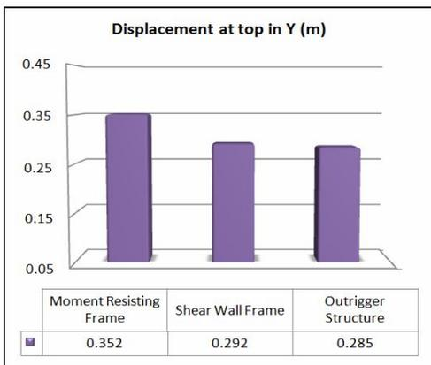
Fig. 8. Comparison of Top Storey displacement in Y dir
