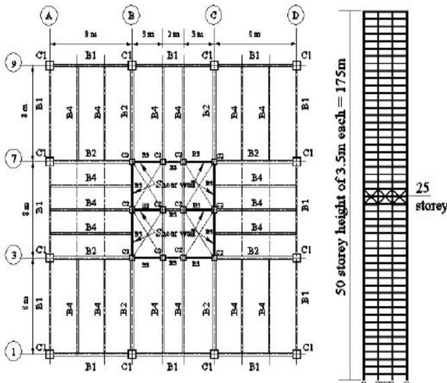
Fig. 5. Outrigger structural system. (Typical floor plan and elevation)
