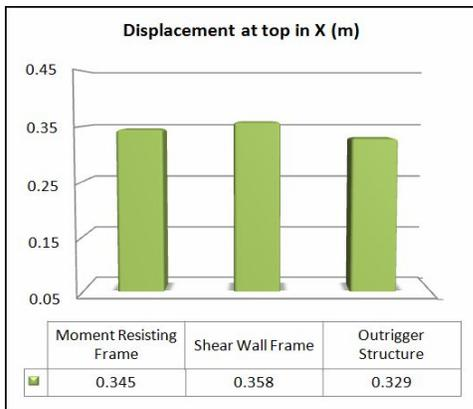
Fig. 7. Comparison of Top Storey displacement in X dir
