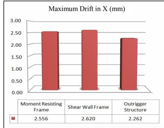
Fig. 9. Comparison of Maximum storey drift in X dir.
