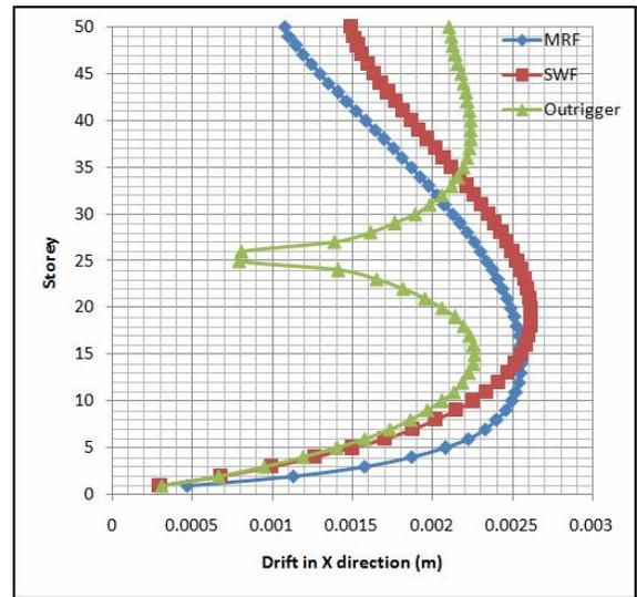
Fig. 13. Storey drift variation along the height in X dir.
