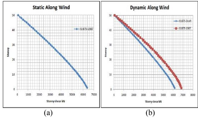
Fig. 1. Storey shear considering along wind loading
