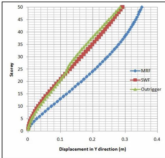
Fig. 12. Storey displacement variation along height in Y dir.
