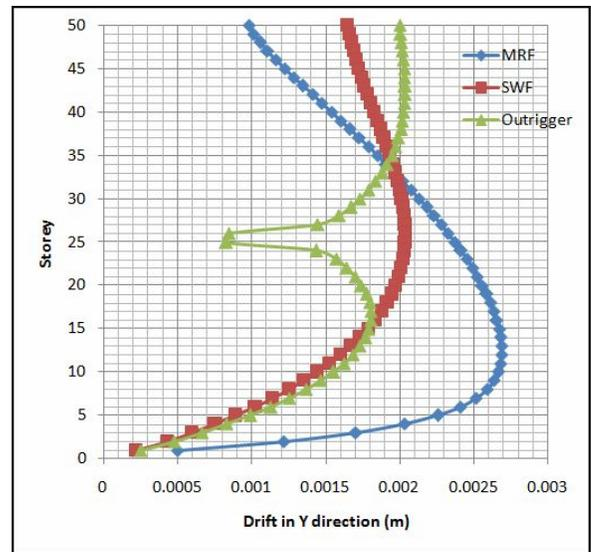
Fig. 14. Storey drift variation along the height in Y dir.
