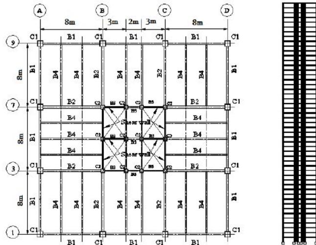
Fig. 4. Shear-Wall Frame structure (Typical floor plan and elevation)
