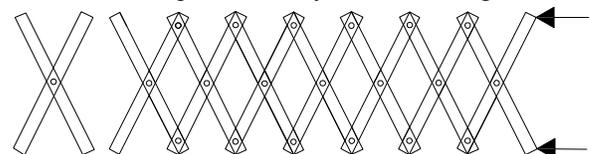
Figure.1A Planar Scissors System
