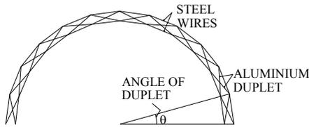
Figure.2 A Scissors Arch System
