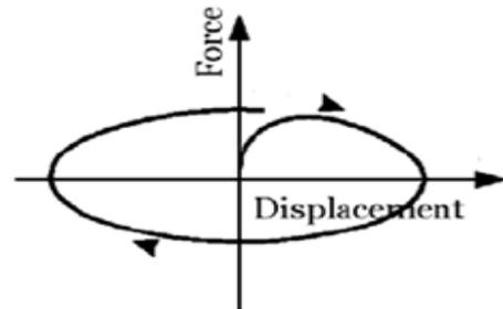
Fig. 4 HYSTERESIS LOOP FOR VISCOUS DAMPER [5]
