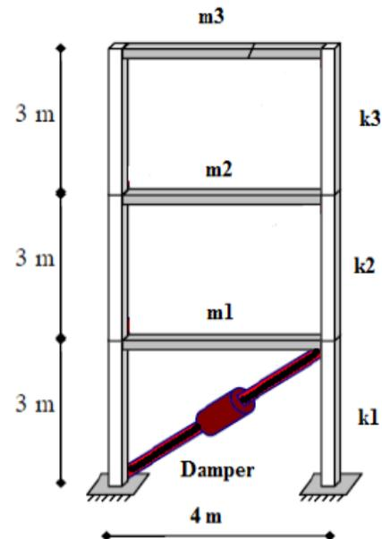
Fig. 8 BUILDING WITH PASSIVE DAMPER AT
