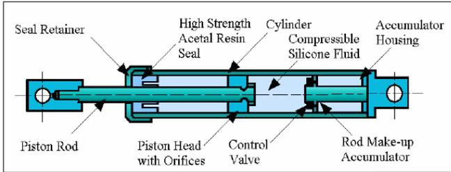
Fig. 2 SCHEMATIC OF VISCOUS FLUID DAMPER [7]
