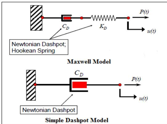
Fig. 3 SIMPLE DASHPOT AND MAXWELL MODEL FOR VISCOUS DAMPER [8]
