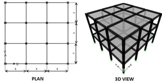
Fig. 7 PLAN AND 3D VIEW OF THE THREE STOREY BUILDING
