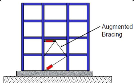
Fig. 1 DAMPER PLACEMENT WITHIN BUILDING
