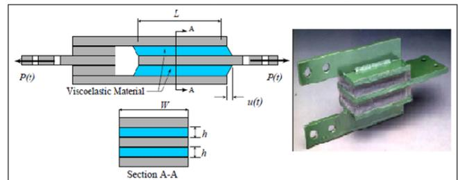
Fig. 5 SCHEMATIC OF VISCOELASTIC DAMPER [8]
