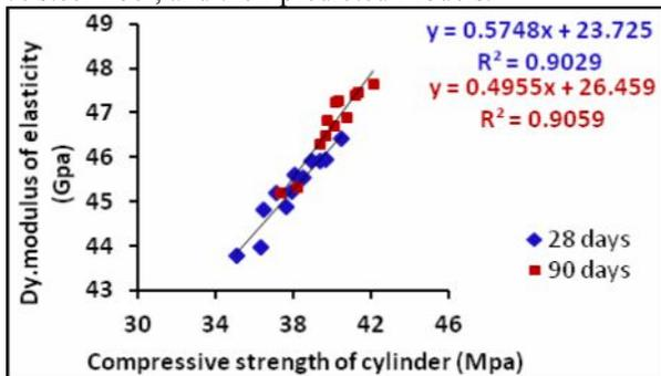
**Figure3.**Relationship between Compressive strength of cylinder ( $f_{cc}$ ) and Dynamic modulus of elasticity (Ed) at 8 % Silica Fume and 0, 0.5, 1.0 & 1.5 % steel fiber, and their predicted Models
