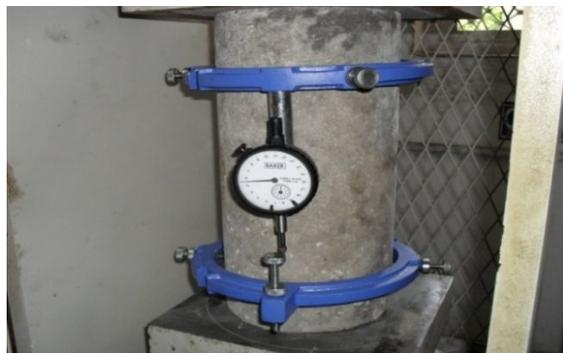
Figure 7. Cylinder Compressive Strength and Compressometer with dial gauge (strain measurement) Test.
