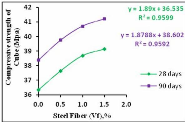
**Figure1.**Compressive strength (Cube) at 28, days of age at 8 % Silica Fume and 0, 0.5, 1.0 & 1.5 % steel fiber, and their predicted Models.
