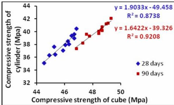
**Figure2.**Relationship between Compressive strength of cylinder and cube at 8 % Silica Fume and 0, 0.5, 1.0 & 1.5 % steel fiber, and their predicted Models.
