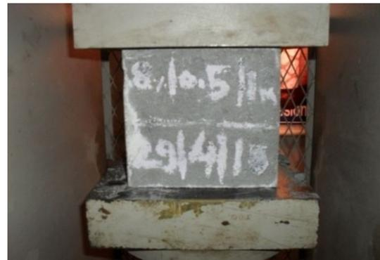
Figure 8. Showed Compressive Strength Test
