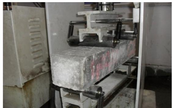
Figure 9. Showed Flextural Strength Test
