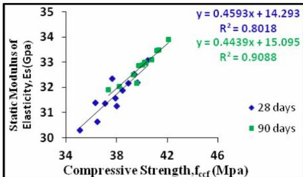
**Figure4.**Relationship between Compressive strength of cylinder ( $f_{cc}$ ) and Static modulus of elasticity (Ed) at 8 % Silica Fume and 0, 0.5, 1.0 & 1.5 % steel fiber, and their predicted Models.
