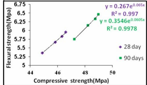
**Figure5.**Relationship between Compressive strength of Cube ( $f_{ck}$ ) and Flexural strength at 8 % Silica Fume and 0, 0.5, 1.0 & 1.5 % steel fiber, and their predicted Models.
