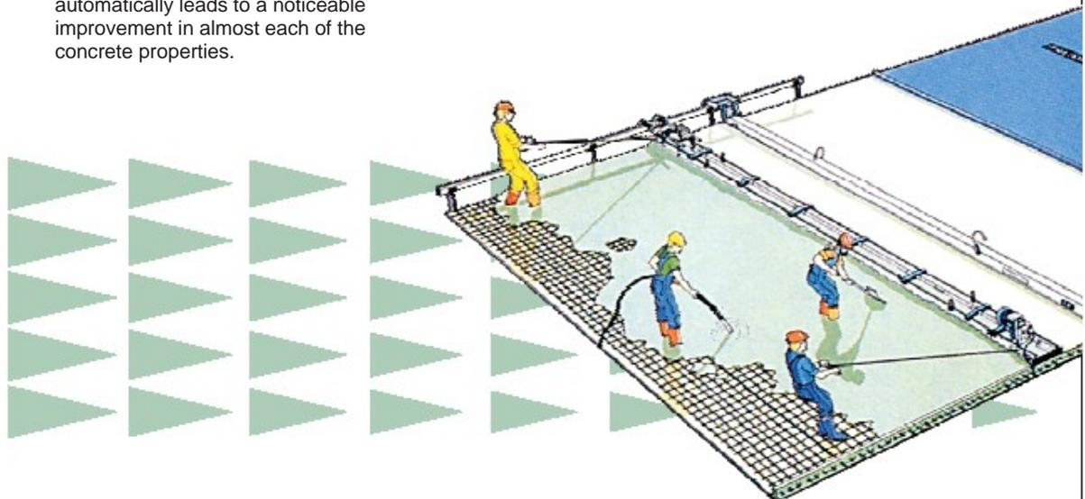
Filter pads are placed on the fresh concrete leaving about 4 inches of fresh concrete exposed on all sides. The Top Cover is then placed on the filter pads and rolled out till it covers the strips of exposed concrete on all sides. The Top Cover is then connected to the vacuum pump through a suction hose and the pump is started.
