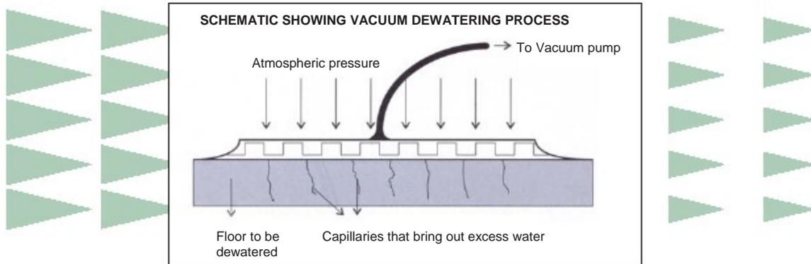
Suction Mat of special grade multilayered polymer sheets alongwith reinforced distance cushions on the Filter Pads ensure sufficient cross-sectional area to squeeze out and remove excess water from the concrete. This design is a prerequisite for effective dewatering.
